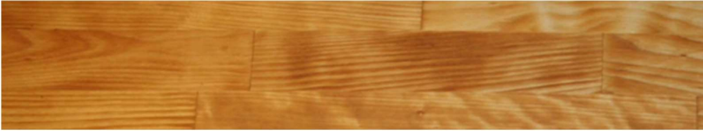
Oil treated board of glued lamellas of birch.
